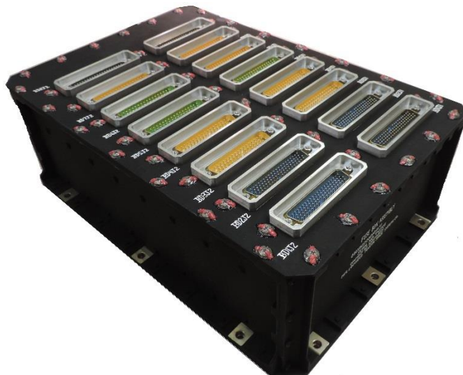
Figure 11-8. A Fuse Board Assembly
