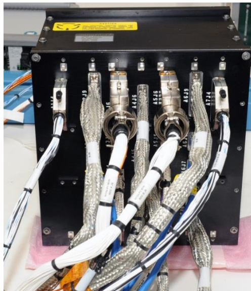
Figure 10-2. The Command and Telemetry Processor (CTP)
