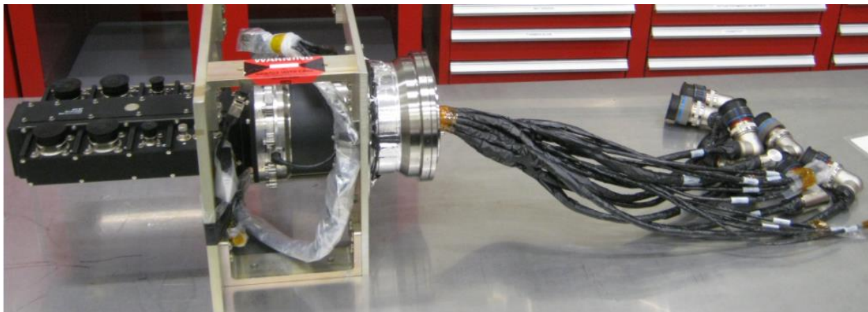
Figure 15-6. Solar Array Drive/Slip Ring Harness Assembly
