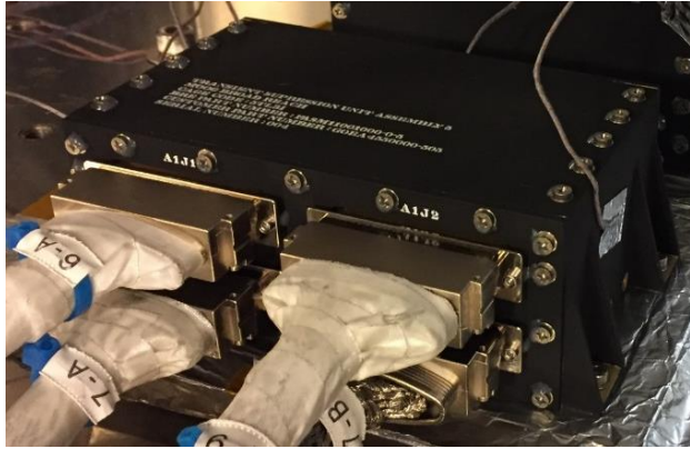
Figure 10-7. Transient Suppression Unit (TSU)
