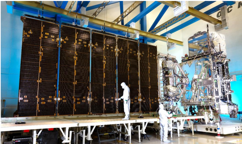
Figure 11-3. The Solar Array installed on GOES-16
