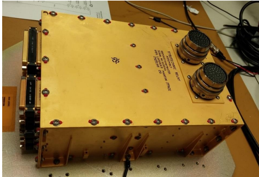
Figure 11-9. The Pyro Relay Assembly
