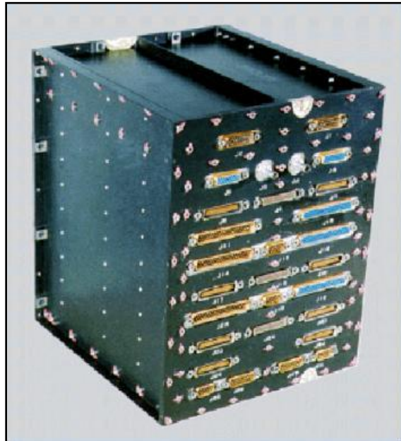
Figure 10-4. Remote Interface Unit (RIU)
