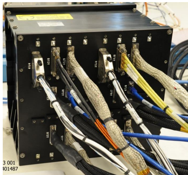
Figure 10-3. The On Board Computer (OBC)
