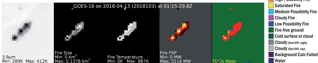
GOES-16 imagery of the Rhea Fire in Oklahoma on April 13, 2018, showing the ABI 3.9 \mu\text{m} shortwave infrared band (left column), and the various outputs of the fire detection and characterization product. From left: fire size, fire temperature, and fire mask. Fire radiative power is shown in colors from black to red for 0 to 1000 megawatts (MW), red to yellow for 1000 to 2000 MW, and yellow to white for 2000-3000 MW. Credit: CIMSS
